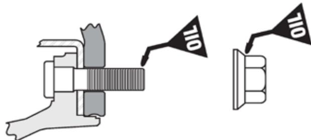
Check (1) if washer freely rotates on nut applying some pressure on the washer towards nut. Fit nut onto the stud and check (2) if the nut can freely rotate by hand turning the nut towards the hub.
